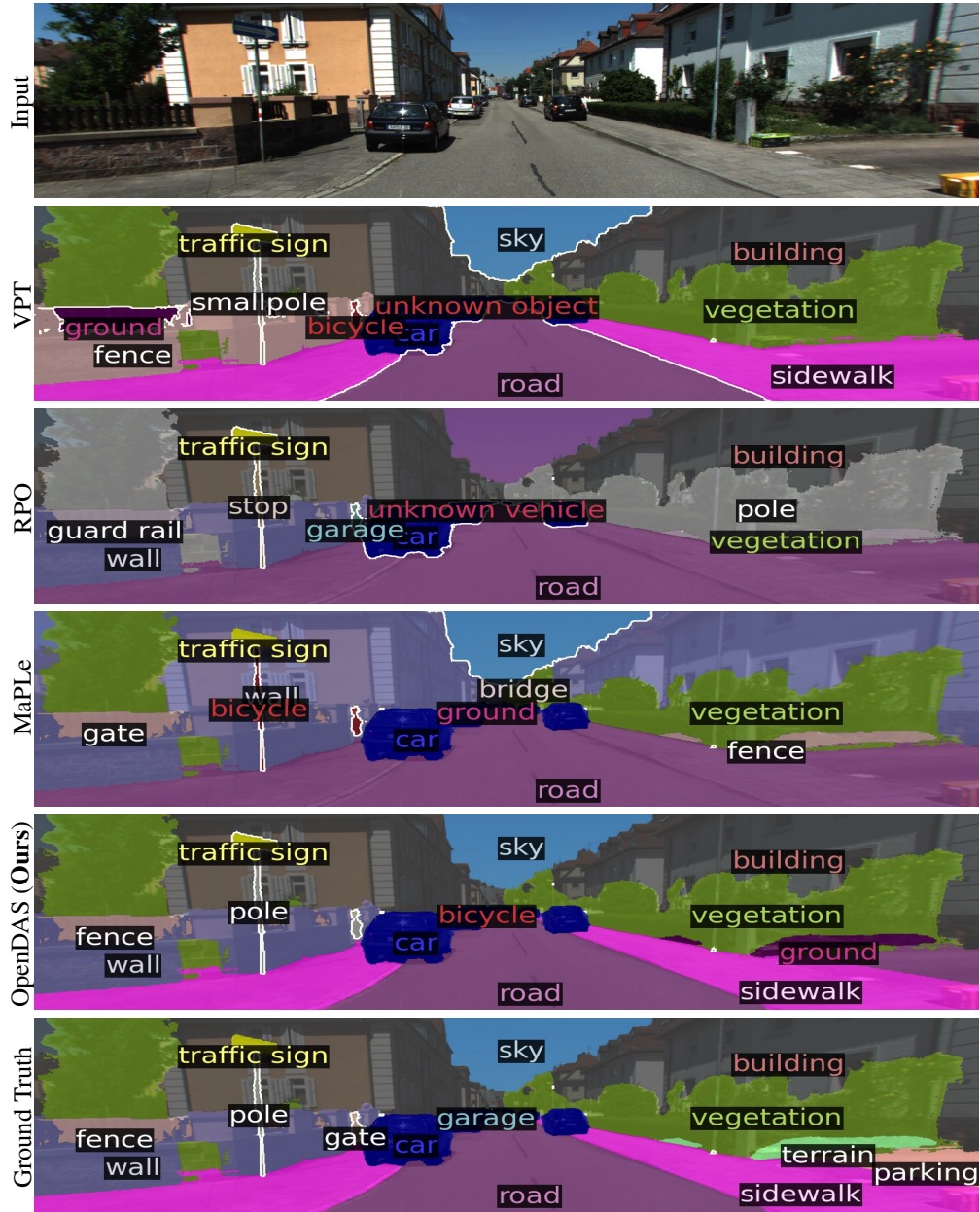
Figure 10: Qualitative Comparison on Segment Classification on KITTI-360 Dataset Liao et al. (2022). We show the predicted object classes with the ground truth masks given on three datasets. The masks are colored based on the class ID. Unlike the existing methods, our model can give the closest match to the ground truth labels understanding the distinction between ‘road’ and ‘sidewalk’.
